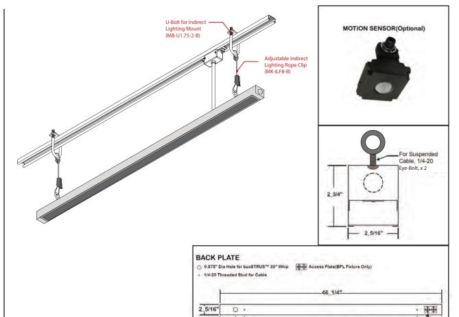
\*Indirect linear fixtures connect to the busway via adjustable cable glide, which is then attached to the U-Bolt (MB-U1.75-2-B).
