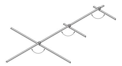
VARIABLE crossovers provide the mechanical connection for building variable angles. The VARIABLE crossover rotates to connect one single-deck length to another single-deck length at any angle. Necessary rotation can be made in the field.
